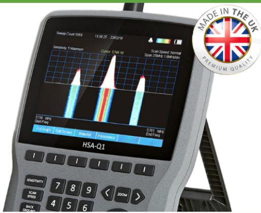
The HSA-Q1 is a handheld RF Spectrum Analyser designed specifically for countermeasures professionals. With a scanning range of 0 to 13.4 GHz in just half a second, it offers unprecedented performance in a truly portable package.
